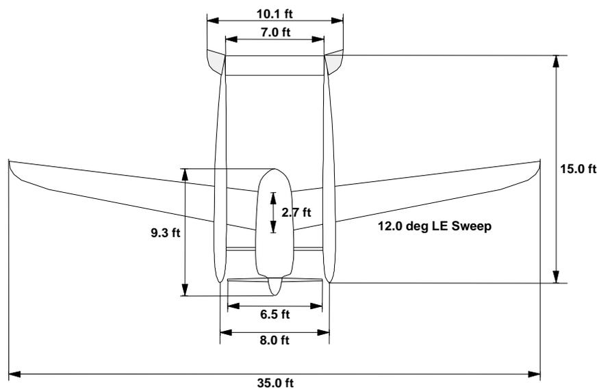
Figure 96. Various views of the MAE tilt-body UAV concept
